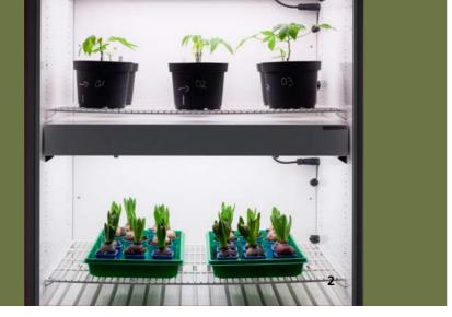
**2** Environmental chamber for simulating different climatic conditions
