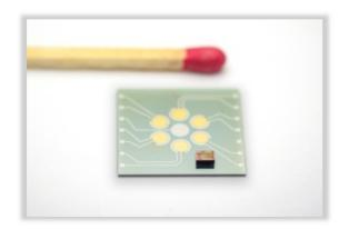
Thanks to an integrated evaluation circuit from Fraunhofer IIS, the biosensor system manufactured by CapSenze can be reduced to the size of a match box.
