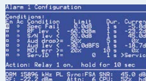
Alarm configuration screen allows enabling and setting of limits for each alarm condition
