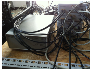
(b) Setup with four USRPs, synchronized via PPS and an external reference clock.
