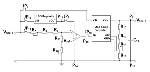
Fig. 4: Schematic for the DC regulated output voltage
