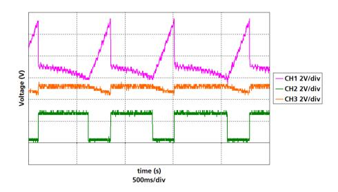
Fig. 7: Steady-state operation of the regulated output voltage on pins X3-1 and X3-2
