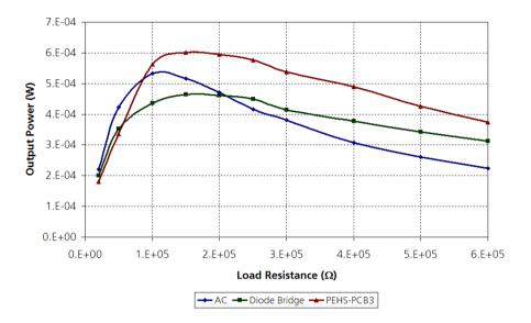
Fig. 2: Harvested power as a function of the load for different topologies employing a piezoelectric element at 16.7 Hz.
