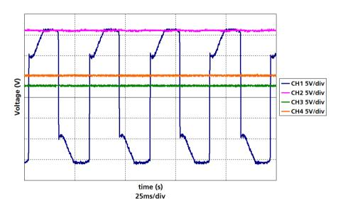
Fig. 6: Steady-state operation of the regulated output voltage on pins X3-1 and X3-2
