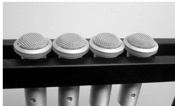
Figure 5: Example for a linear array of four microphones
