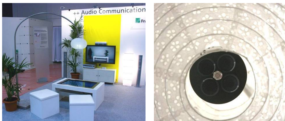
Figure 3: Microphone array embedded in arc-lamp as shown at IFA 2009 (left) and detailed look from below showing the four omnidirectional microphone capsules (right).
