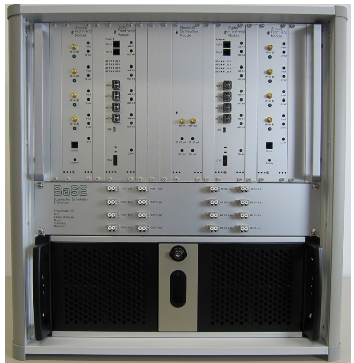
Figure 3: BaSE receiver setup without antenna
