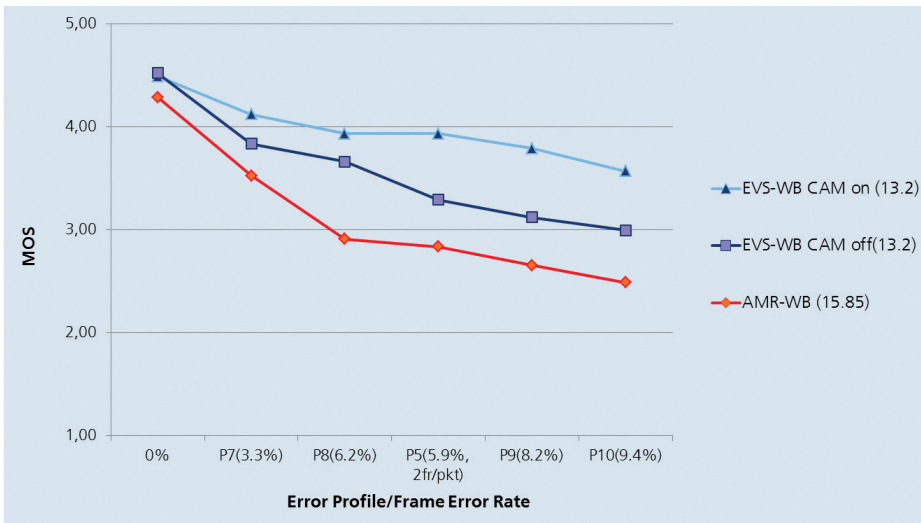
Figure 4: Robustness comparison between AMR-WB and EVS (CAM on and off). EVS maintains its high quality even at a frame error rate (FER) of up to 3% (CAM off). EVS' performance at a FER of 6.2% is comparable to AMR-WB's performance at a FER of 3.3%. The same comparison applies for CAM enabled EVS at 9.2%.
